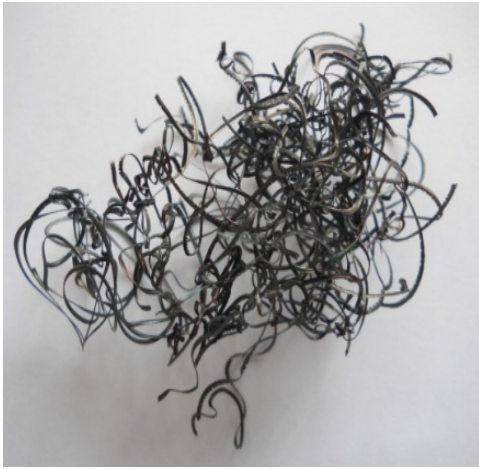
Long ribbon type chip in case no.(24)
